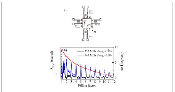
Figure 1. (a) Top view of the Hall bar contact pattern and SAW transducers. The two sets of transducers (IDT-1 and IDT-2), which are connected pairwise in parallel, transmit SAW along perpendicular crystal axes at different frequencies. (b) Changes in SAW phase, measured in a time window centered on the  $\,$ rst SAW arrivals, show the increase of SAW velocity coincident with Hall-resistance plateaus at integer  $\,$ lling factors. Note that the scaled  $\,$ R $_{\rm Hall}$  axis is logarithmic.
