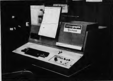
HOT AND COLD - Formidable-looking device in upper picture is a linotype machine, on which hot lead is cast into type. Lower picture shows the CG7200, a device which prints headlines in cold type. "Orient" used hot type process for years, but has now changed to cold type. (See column on Page 4).
